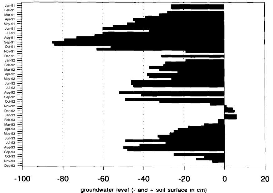
**Fig. 2.** The fluctuations of the groundwater level at location PU of Fig. 1 (A.C.D. Ertsen, pers. comm. 1994).
